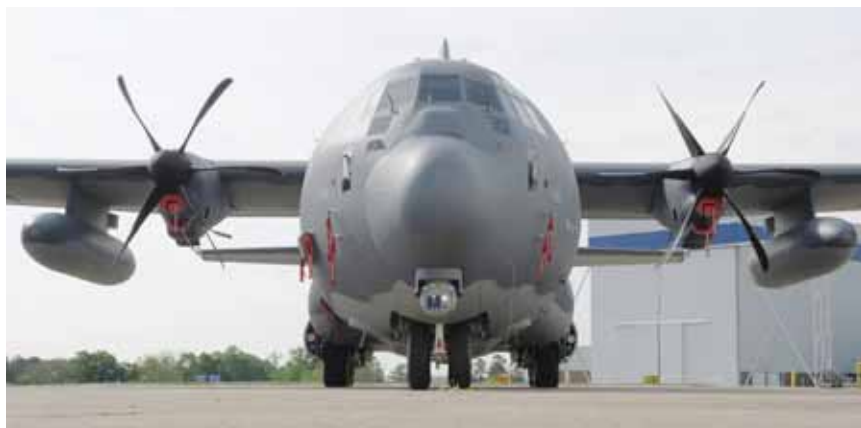
The HC-130J is the US Air Force's new combat tanker and personnel recovery aircraft
