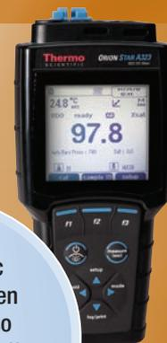
Orion polarographic dissolved oxygen probes are also available, which offer compatibility with the Orion Star A323 meter.
