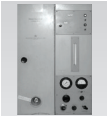
The Model 154-B Gas Chromatograph. The column oven is behind the door on
