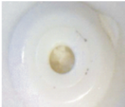
Visible image (x4 objective) of the blockage taken using the camera of the RamanMicro 200.
