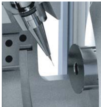
The patented angled design of the Flexar SQ 300 MS probe enhances the desolvation process and provides charged molecules with additional momentum to reach the capillary entrance.
