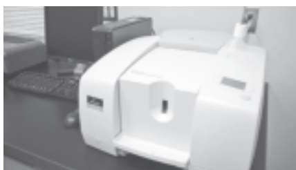
Spectrum 100 FTIR with Plug-n-play DRA accessory
