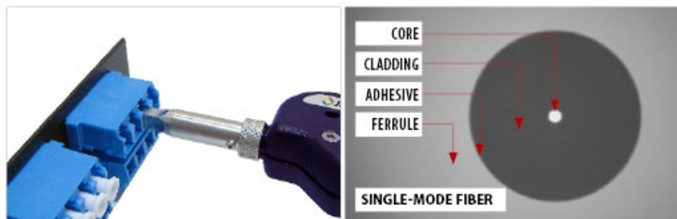
Figure 7. Microscope inspection through the bulkhead/adaptor connector
