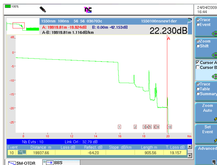
Figure 16. Cascaded splitter network test from OLT, without launch cable
